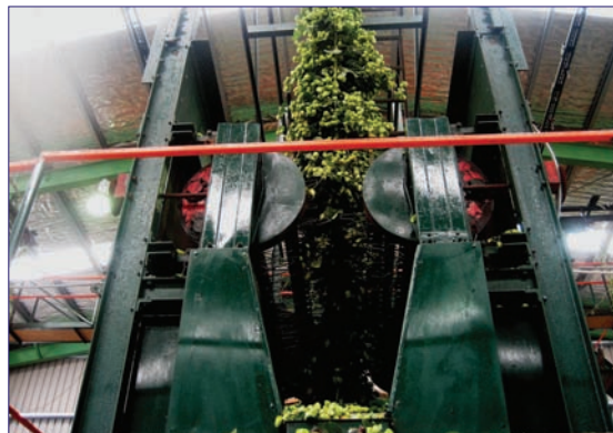
A Bruff hop picker in operation at the NZ Hops plant
